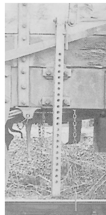
NER 20Ton wood hopper wagons had long travel brake guards.
