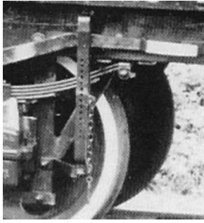
Standard RCH type with axleguard tie with a central tab.
