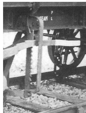
Later GWR ratchet brake guard with axleguard tie.
