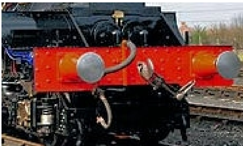
A GWR King showing the common way that screw couplings were stowed. Note the vacuum pipe and steam heating pipe (?) to the left of the coupling hook.
