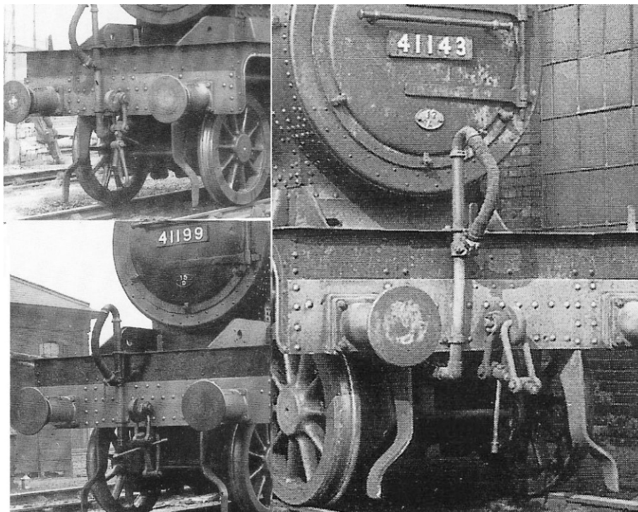
Other ways of stowing a screw coupling: 1- where the coupling loop is retracted 2- where the coupling loop is folded backwards and upwards 3- where the bottom loop has been hooked over the coupling hook.
