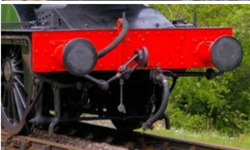
However on this "2251" class engine a steam heating pipe lies to the right of the coupling hook and the screw coupling has been stowed to the left.
