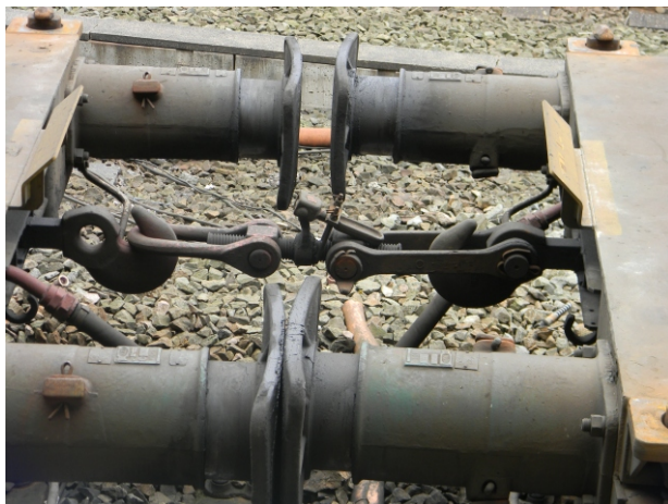
A modern coupling with two screw threads fitted to container wagons, there is no unused coupling link - these wagons are kept in sets. Note the projection of the hook beyond the buffer beam in conjunction with UIC type long buffers. The hooks are able to slide along slots in the buffer beams which give lateral flexibility.
