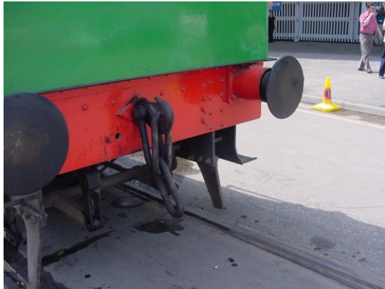
A shackled three link loose coupling, where the coupling has been looped over the drawbar hook.
