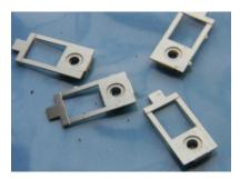
There is a relieved section on the inner layer which was added to assist in mounting some 7mm scale axle bearings. The folds occur in the standard way - towards the half etched line
