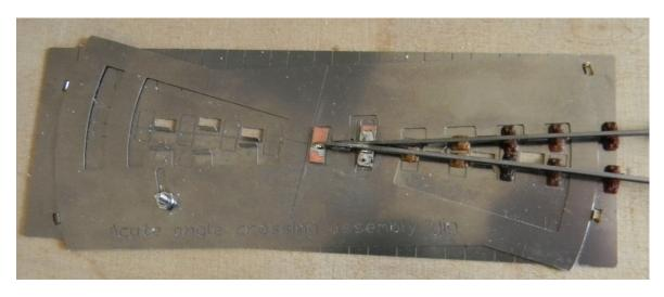
\*\* For smaller crossing angles it will be better to use 3 PCB Strips under the nose not two, although the wing rails need not extend the extra distance.
