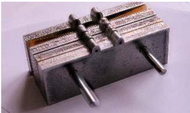
The tool for shaping round buffers into an oval shape was laser cut with packing pieces etched in brass.
