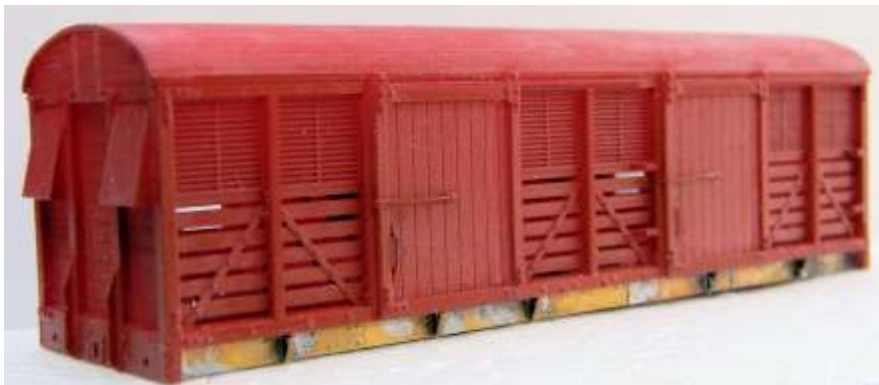
The Stoke 5D modern resin printed LMS fish/slatted milk van in a red primer with the beginnings of an etched chassis.
